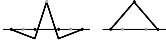
Figure 4: Wavelet and B-spline scaling function.
