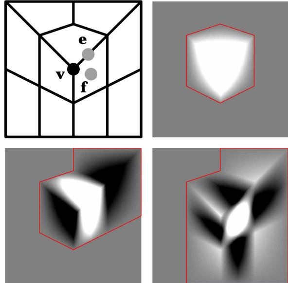
Figure 6: Basis functions near an *extraordinary vertex* of valence three. Scaling function (top right),  $\mathbf{e}$  wavelet (bottom left), and  $\mathbf{f}$  wavelet (bottom right). Dark regions correspond to negative and bright regions to positive function values.
