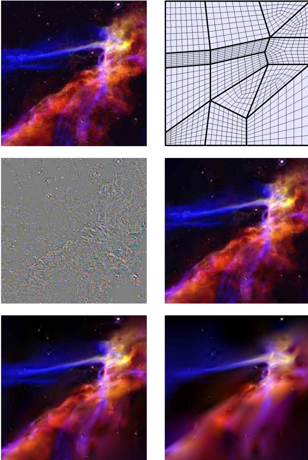
Figure 7: “Cygnus Loop” Hubble image. Top left: original, resampled image on tessellation  $T_7$  (217921 samples); top right: tessellation  $T_0$  and three levels of subdivision; middle left: our wavelet transform (the coefficients are scaled by 10 and a grey level is added); middle right: reconstruction from 10 percent of coefficients; bottom left: 1 percent of coefficients; bottom right: 0.1 percent of coefficients.
