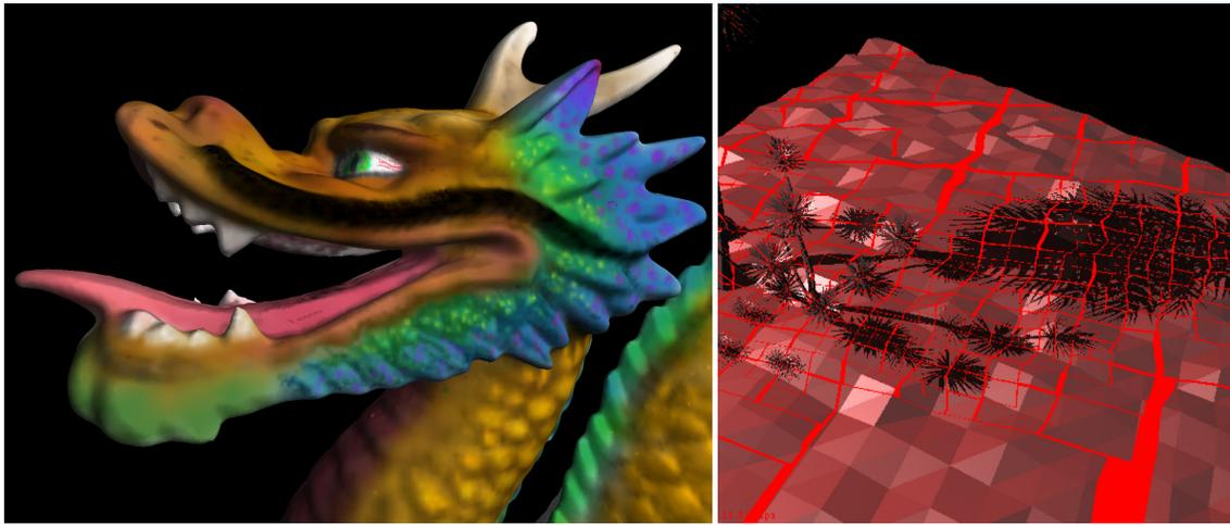
Figure 2: At left, an 817k polygon model with paint stored in an octree with an effective resolution of  $2048^3$ , using 15 MB of GPU memory stored in a Glift 3D adaptive multiresolution data structure that supports quadlinear filtering on the GPU. At right, a visualization of an adaptive shadow map stored in a Glift 2D adaptive multiresolution grid on the GPU.
