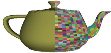
Figure 1: Flat-shaded OpenGL renderings of Reyes-subdivided surfaces, showing eye-space grids generated during the Bound & Split loop.
